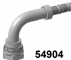
BURGACLIP - connection fitting with a female metric thread, type DIN 3865, 24° cone, light series
