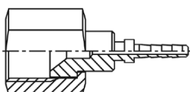
UNF female thread, SAE type, 45° cone, (1/12 - brass, 5/32 - steel)
